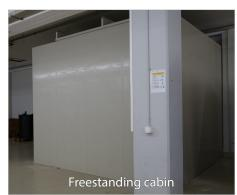
Plastic polypropylene (PP) is often used in constructions because it is chemically resistant and is always easy to clean. Due to these properties, factories often use PP cleaning or spray booths for a broad spectrum of purposes. Roth Kunststoftechniek made a cleaning cabin of 3 m x 4 m x 3 m with Paneltim® panels made of PP copo. The cleaning
